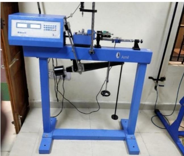
**Fig:2 Direct shear apparatus setup**
