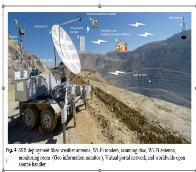
Fig. 4 SSR deployment like weather antenna, Wi-Fi modem, scanning disc, Wi-Fi antenna, monitoring room (Geo information monitor), Virtual portal network, and worldwide open source handler
