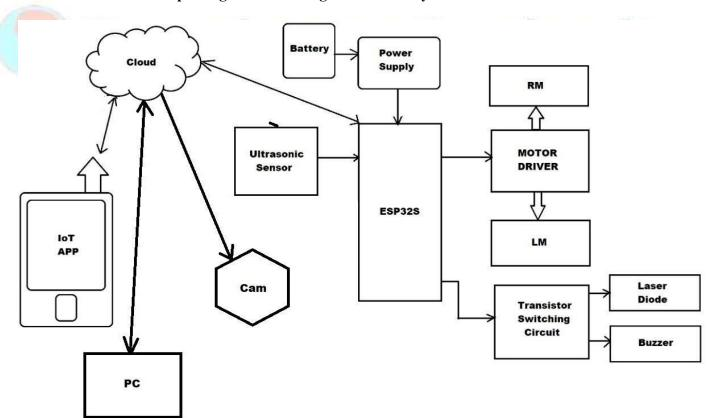
Fig 1: Stream robot schematic representation
