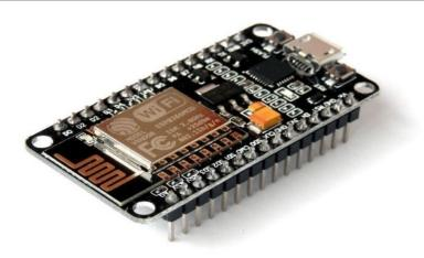
Fig 2: Node MCU -ESP8266
