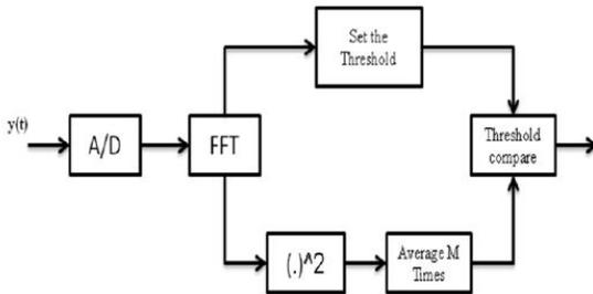
**Fig 4: Digital implementation of an energy detector**
