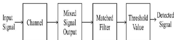
**Fig 2: Common Blocks for Matched Filter Detection**
