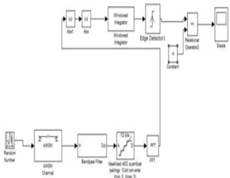
**Fig 5: Simulink model for Energy Detection**
